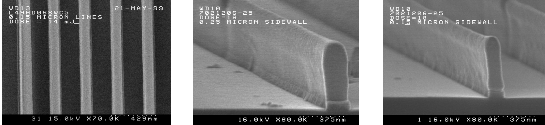
Figure 19: Top down view of 0.15 μm nested lines, side view of 0.25 μm isolated line, side view of 0.15 μm isolated line
